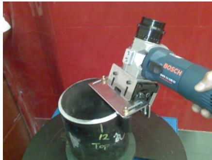
We have seen increased sales in the **Chamfo** plate and pipe bevellers so far this year. These bevellers offer a low cost, yet precise method of beveling plate and pipe for weld preparation and there are 3 models in the range. The largest beveller, which is still a hand held tool, allows for putting a 35° weld bevel on steel, stainless
