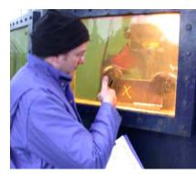
them on the possibility of wet welding some high CEV steels. We are pleased to advise that by using procedures developed by our resident welding engineer David Keats we have shown it has been possible to weld this material, using our Hammerhead Cr-Ni-Mo (stainless) electrodes.
