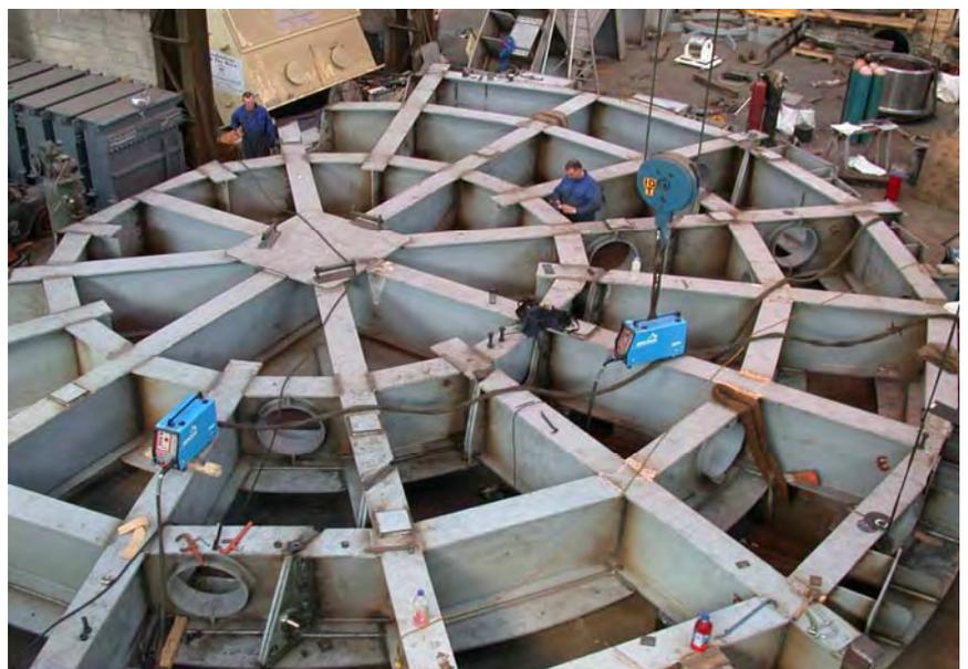
section (up side down) which has to be built in sections so it can be transported. When completed and fitted onto the vessel the total fabrication weight will weigh over 2000 tons; that's what you call a lot of cable reeling!
