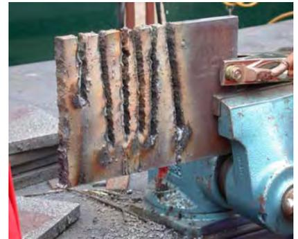
conducted at **NHC's** facilities in Aberdeen, utilising their 11M wet tank. Two RBG divers where shown by David Keats how to use the product through a brief practical demonstration which was also witnessed by Shell. The photo shows the various cut lines produced by the divers, while practicing in air, using the **Swordfish** electrode, prior to diving.
