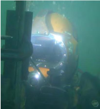
multipass vertical-down welding techniques for their divers, using our **Barracuda** electrodes. Divers being successfully qualified under our **UKAS/SAFed** accreditation to BSEN ISO 15618-1: 2004. All training was conducted at **FJ. Marine** base in Merseyside; which provides excellent facilities for both wet and dry welding and is ideally located for companies on the West coast; cheers Fred.
