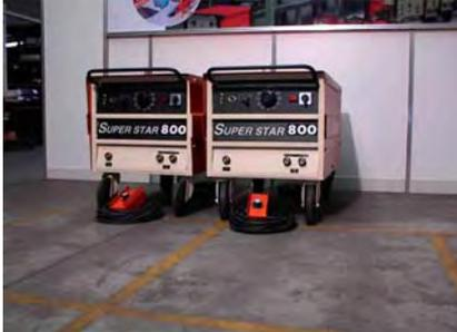
range of welding transformer-rectifiers. These popular machines are modified for use offshore being fitted with stainless steel panels and specially designed fans/intakes to reduce problems caused by dust. The range available starts from 200 and goes up to 800 amps.
