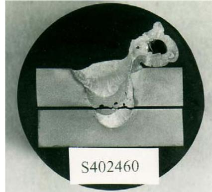
*Shows a wet-spot weld and 'flash' (excess material) cut through the centre and macro polished (x 2 mag)*
