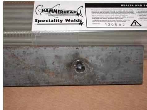
*Plate shows this piercing effect and the hole created by the 1<sup>st</sup> high current.*
