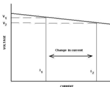
A typical ‘flat’ characteristic for MIG welding.
