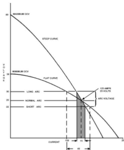
A typical 'drooping' characteristic curve for MMA welding.
