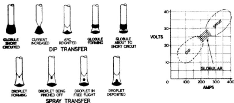
Shows dip and spray transfer mechanism and the current/volts necessary.
