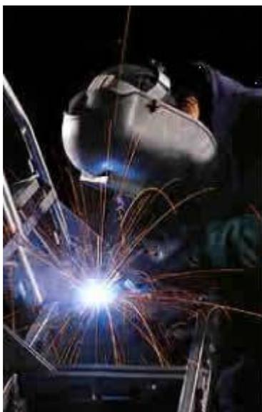
A more accurate term might be described as ‘semi-automatic’, meaning the arc is ‘self-adjusting’. Any variation in the arc length produces a change in the ‘burn-off’ rate allowing rapid re-establishment of the original arc length.
