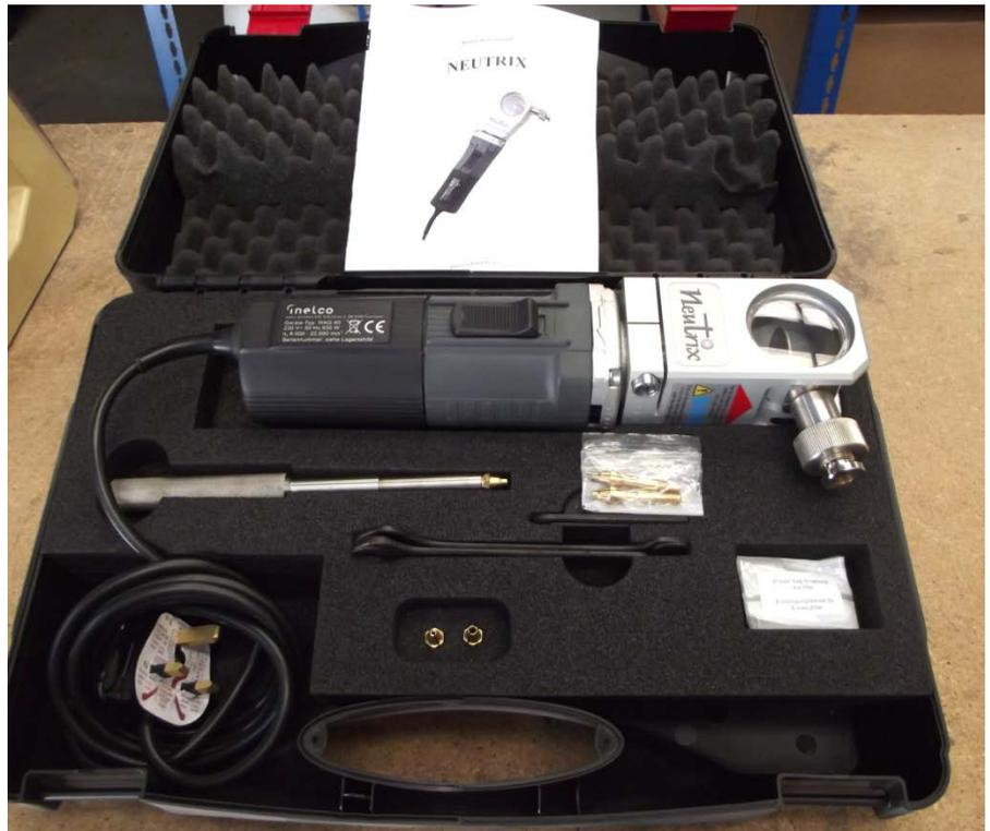
their welding operator certification, we are pleased to have supplied them with the portable enclosed tungsten grinder. The **Neutrix tungsten grinder** is not only essential in order to produce a precisely ground tip, which is required when using automated welding systems, but also ensures the harmful thorium dust is kept away for the operator while grinding. If you would like to learn more about this tool, please contact our sales team.
