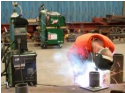
welding trails using **Barracuda Gold**. We were asked to advise them on all welding issues and produce appropriate WPS. The welding is to be conducted for **Eilat Ashkelon Pipelines**, an Israeli company, and will involve welding a new flange to an existing pipeline.
