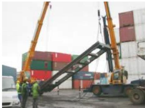
examination/certification services, and had it operational in less than four days. The mast you can see in the picture is where the cracks were located; these masts weight in just shy of 10 tonnes. Trucks operate in harsh conditions and are lifting containers all day over rough
