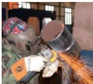
Portland based **Dive Technologies** requested our assistance to advise on new British/European welding codes and standards, and formally qualify their team of welders for a forthcoming contract. The team needed to qualify for butt welds in steel pipe and plate in the 6G and 3G positions, using the Manual metal Arc (MMA) process. Kirkwall based **Leask Marine contracted** us to provide training for their divers in both wet and dry stick welding.
