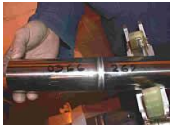
Completed orbital weld on 50x1.6mm stainless
