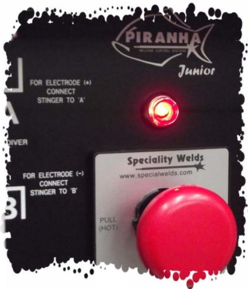
If you are using the **Junior** model (no meters fitted) then still ensure all cables match like for like, as detailed above. To test whether the indicator light operates correctly, pull the red on/off knob to make a live (HOT) connection; the indicator lamp will now illuminate. By pushing the red on/off knob down (making it cold) the indicator light will extinguish. This procedure now ensures the correct set-up and you are ready to connect the welding cables to the diver.
