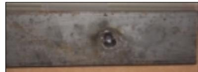
Plate shows this piercing effect and the hole created by the 1st high current.
