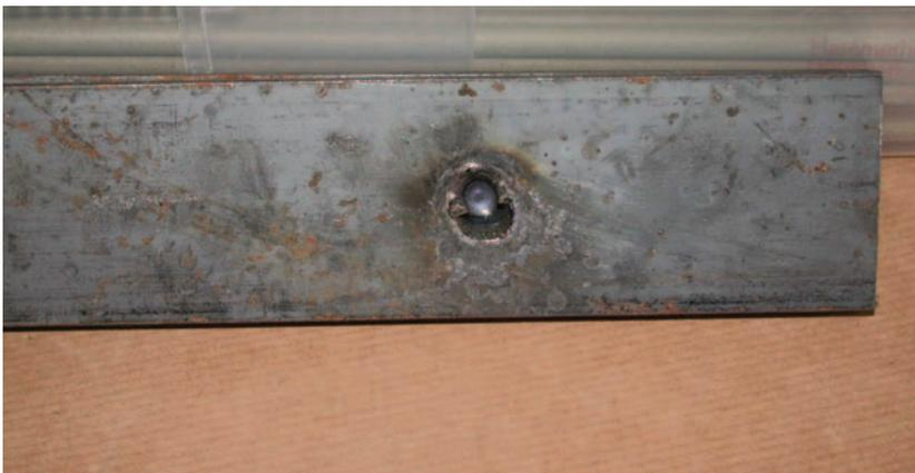
Plate shows piercing effect and the hole created by the first high current
