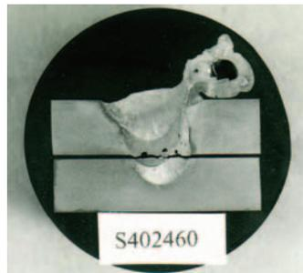
**A spot weld and flash cut through the centre and macro polished**
