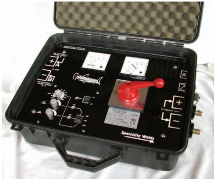
Control system housed in 400A safety switch/control unit
